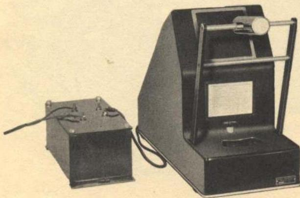
*A special transformer maintains the constant intensity of the lamp, an essential feature in a photo-electric instrument.*
